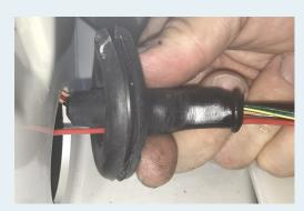
The other end of the cable you have installed has a spade connector. This cable must be fed into the vehicle and connected at the fusebox.
