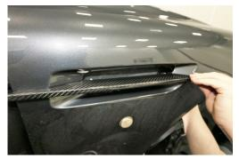
Position an adhesive pad on the carbon strake on the trailing edge and remove the protective backing strip from the sticky pad.
