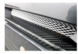
Carefully open the door paying very close attention to the clearance between the pip and the wing trailing edge as shown in the picture (left). The pip must not come into contact with the wing.
