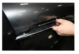
Withdraw the chrome side strake. The ends of the OEM side strake may be held on the bodywork by an adhesive strip. It is safe to simply pull the side strake off but you must clean off all residual foam from this adhesive strip before continuing.
