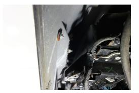
There are 4 nuts holding the side strake on the wing.
