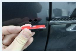
Clea off any adhesive residue left from the chrome pip. Isopropyl alchlcohol is really useful to prepare surfaces for good adhesion and cleanliness.
