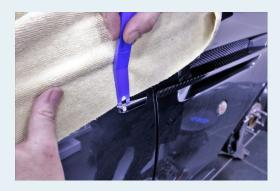
Using the microfibre cloth and trim tool (available at www.divinatech.com), pry off the door pip. Be very careful not to dent or scratch the paintwork. Use slight and even pressure to work the sticky pad that holds it until it comes off.
